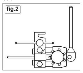
4.1.8. After the pipe has been prepared as instructed above, ensure the tube nut is fitted to the pipe. Pass the pipe through the rear of the die until the prepared end is flush with the front face of the die. Ensure that both halves of the die are contacting the die stops (fig.2). Swing the locking plate into position and tighten the clamping screw. Check that the position of the pipe and die are still correct.
